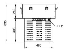
D = Drain El = Electrical inlet (power)
